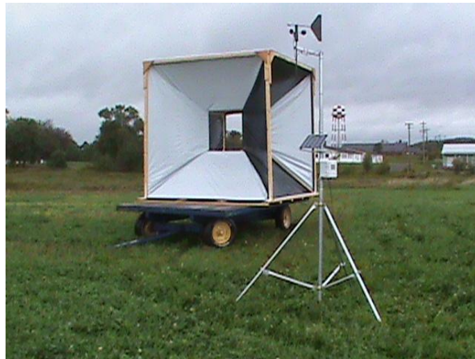
Figure 5. Image of field test with cube and free standing wind speed sensor.
